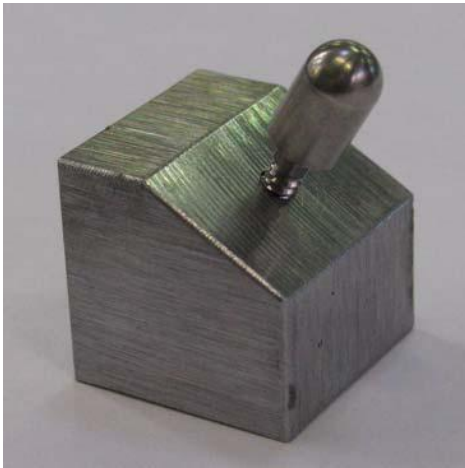
Fig.4: Implant with hemispherical member mounted on the specimen holder
