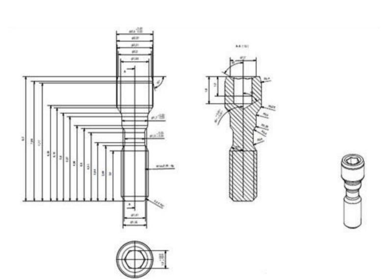
Technical drawing of the connection screw of dental implant system JDEvolution
