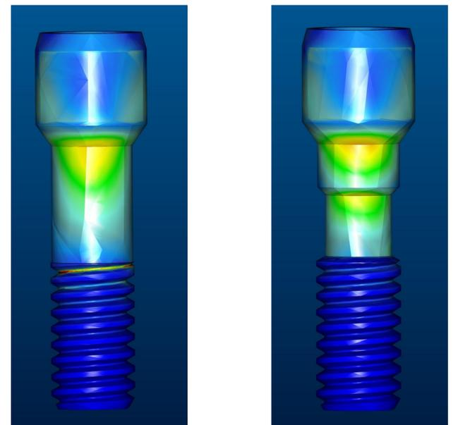
Tensional state of the two screws design evaluated: on the left traditional screw design, on the right JDEvolution design.
